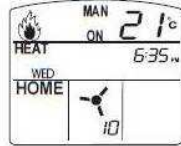
Normal display with heater running in MANUAL mode.
